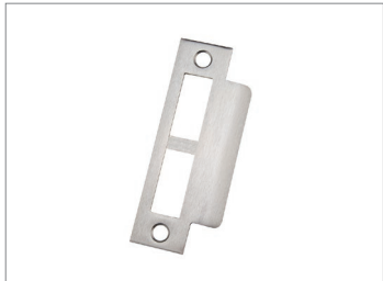
Brass Standard Strike Plate 1 \frac{7}{8} " wide x 4 \frac{7}{8} " high Supplied with Mortise Locks unless door thickness is specified as 2" or greater
